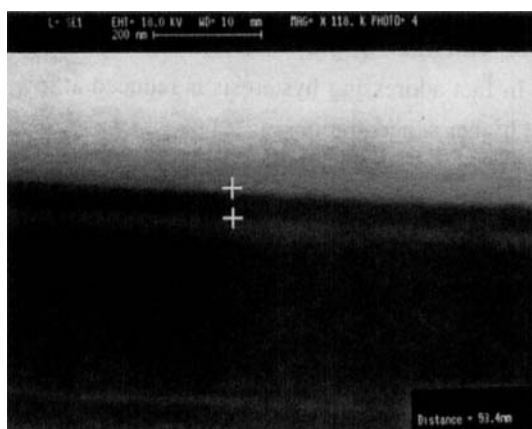
FIGURE 1 Scanning electron microscope of a nylon film deposited by spinning. The film section appears dark, due to lack of gold.
